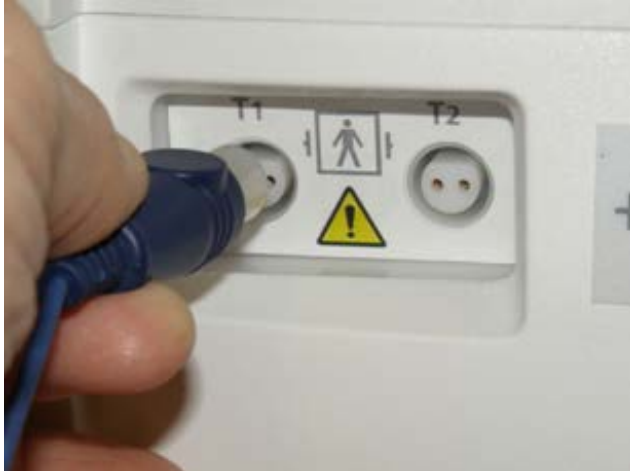
Figure 4.50. Temperature Probe Connections
