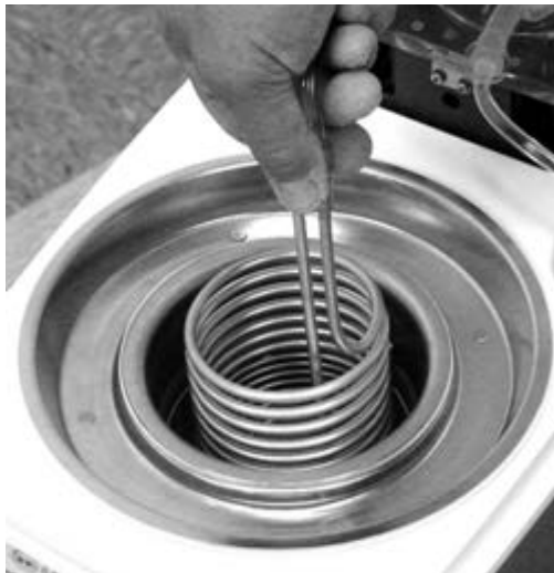
Figure 4.39. Installing the Heat Exchange Coil
