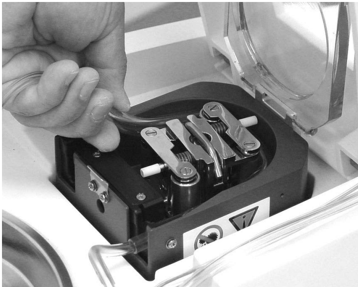
Figure 4.43. Pump Tubing Installation
